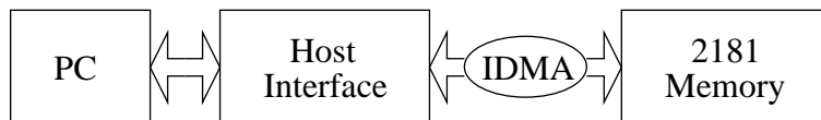
Figure 5: Access to the memory of the root processor via the host adapter
